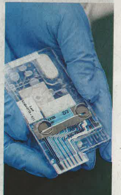
Racer Technology's Mr Koh gets on the fast track in the medical technology industry with the firm's diagnostic tool, a microfluidic chip (right), which can produce blood-test results in minutes which would otherwise take up to two weeks in a lab. PHOTOS: YEN MENG JIIN
